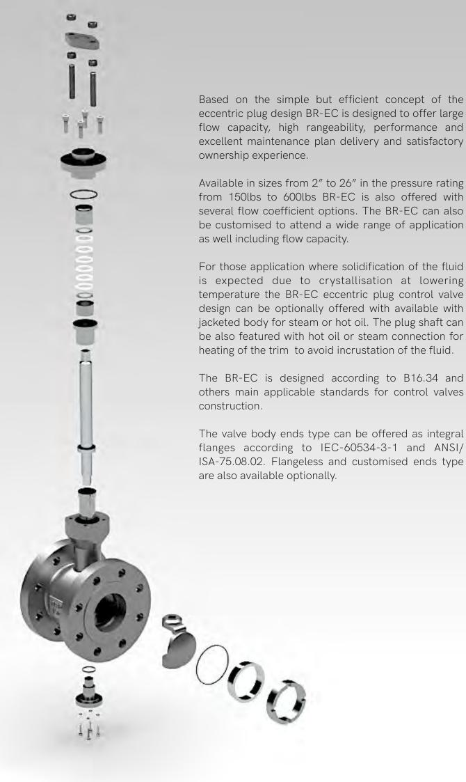
Offered with an advanced packing system The BR-EC model is also certified for low fugitive emission services according to ISO 15848 - and Shell MESC 77/312. As standard when the GreenSeal Supermax packing is offered the BR-EC is certified for low fugitive emission endurance class CC1 up to 200 degC, tightness class BH.
